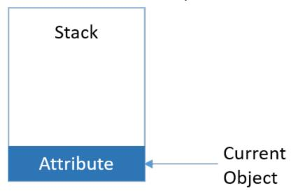
Now a macro is used that pushes the Attribute object's owning Entity onto the stack. The stack will now have two entries, with the Entity being the current object.
